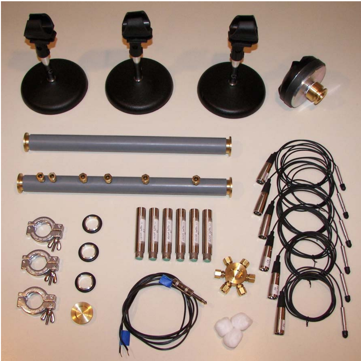
Figure 2.2. Minimum hardware for reflectometry. Starting at the top, the photo shows three waveguide stands, a compression driver, a straight section, and a six-station microphone section. Below the microphone section on the left are three coupler clamps, three seals with o-rings, and a closed end. At center are six buffer amplifiers, and below them is a cable for the compression driver. To the right is a six-station calibration cell, three cotton balls, and six microphones. Each microphone has a black rubber cap over the sensitive end for protection.
