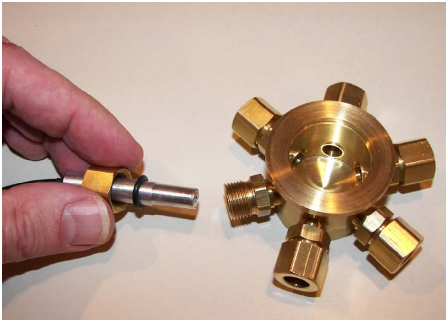
Figure 2.5. Assembling the calibration cell. Place the threaded cap and the o-ring on the microphone before inserting it into the calibration cell.
