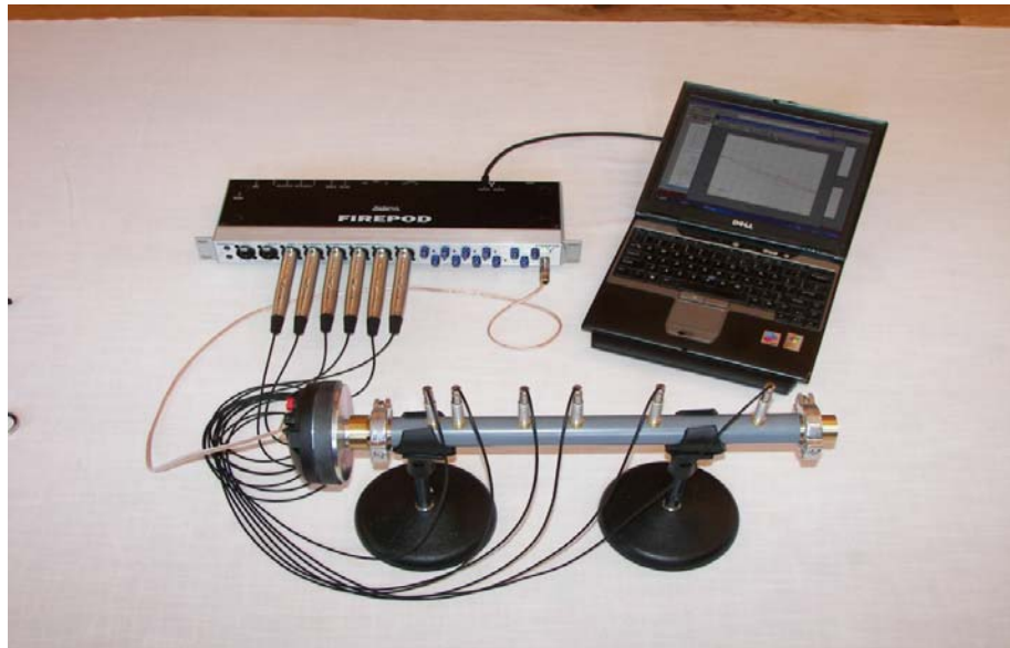
Figure 3: In the top left is the digitizer with six buffer amplifiers leading from each microphone. The AVNA is shown with a closed end attachment in the foreground atop two stands.
