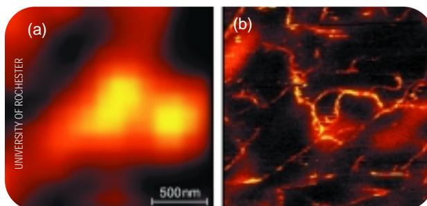
Images of carbon nanotubes on a glass substrate compare conventional microscope image (a) with near-field Raman technique (b).
