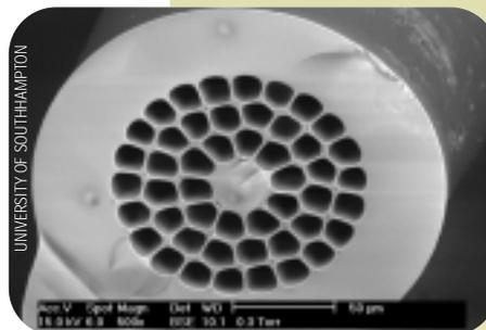
A JAC fiber has a 10- $\mu\text{m}$  core centered within a 28- $\mu\text{m}$  Yb-ion-doped cladding layer, which is in turn surrounded by three layers of "holey" silica and then a silica outer shielding.
