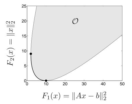
example for  $A \in \mathbf{R}^{100 \times 10}$ ; heavy line is formed by Pareto optimal points
