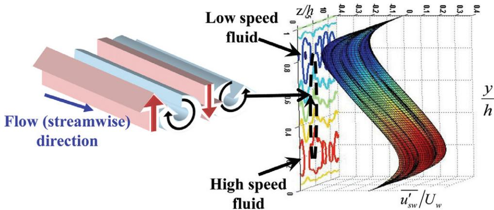
Fig. 3. Cartoon of streamwise elongated structures with surface plot of 2D/3C simulation results.
