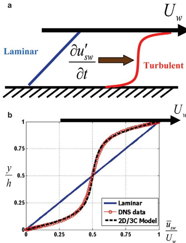
Fig. 4. (a) The laminar and blunted or “S” shaped turbulent velocities profile for plane Couette flow driven by motion (at velocity  $U_w$ ) of the top plate. (b) The 2D/3C simulation captures the change in profile from a laminar initial condition to a turbulent mean velocity profile.
