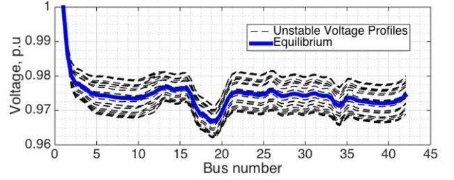
Fig. 3: Oscillation in voltage profile when all inverters operate.
