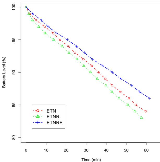
Fig. 6: Battery Consumption for Different Routing Schemes
