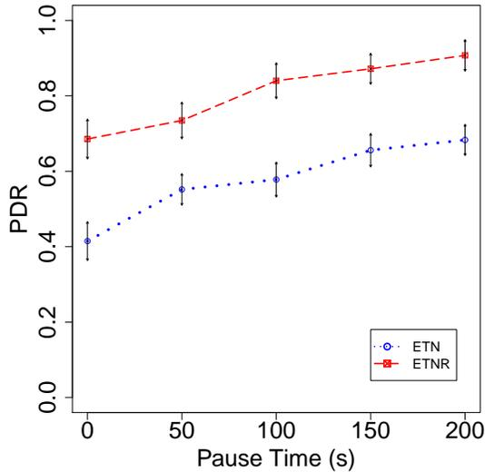
Fig. 4: Packet Delivery Ratio Comparison for Locally Reactive Routing
