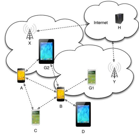
Fig. 1: System architecture of the hybrid cellular-MANET
