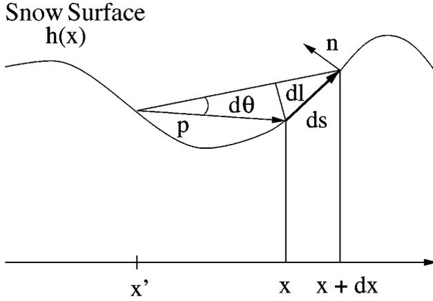
FIG. 5. Schematic of the ablating snow surface. Scattering from the point  $x_1$  to the interval between  $x$  and  $x + dx$  depends on the angle  $d\theta$ . The vector  $\mathbf{p}$  points from  $x_1$  to  $x$  and the increment  $d\mathbf{l}$  is normal to  $\mathbf{p}$  such that  $d\theta = d\mathbf{l}/p$ . The vector  $\mathbf{n}$  is normal to the surface at  $x$  and  $d\mathbf{s}$  is the increment along the surface between  $x$  and  $x + dx$ .
