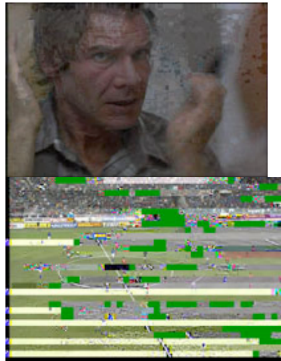
Figure3. Movie frame showing effect of perceptual attack on encrypted quantizer_scale_code (fixed at 5 in the reconstruction) (top) and sports frame showing effect of 20% encryption of macroblock_type (bottom).
