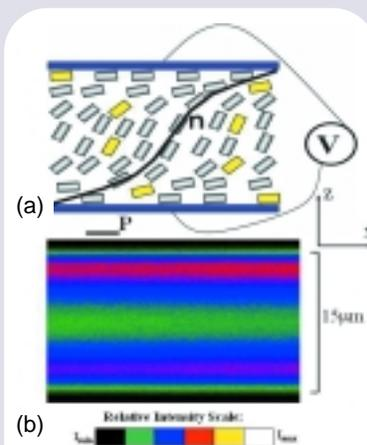
A vertical cross-section shows an LC cell undergoing the Frederiks transition under an applied electric field: the director field ( $n$ ) describing the average orientation of LC molecules (a) and the FCPM texture visualizing this director field (b).
