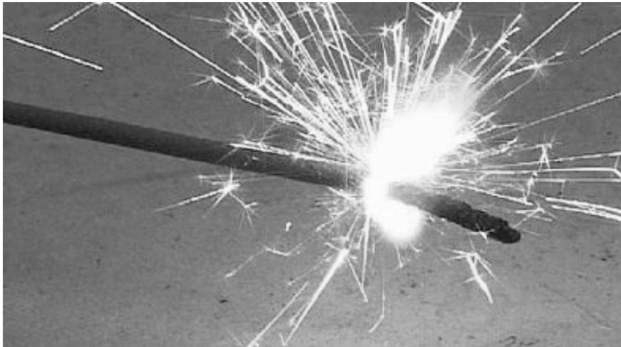
>Fig. 2. Sparklers are a form of solid rocket propellants in composition and they burn at about the same rate as Space Shuttle Solid Rocket Booster propellant, i.e., less than about 0.2 inches per second at atmospheric pressure. A sparkler takes about a minute to burn from one end to the other. If it burned at the speed of the *Hindenburg* fire, a sparkler would burn in a flash lasting only about 0.04 seconds.
