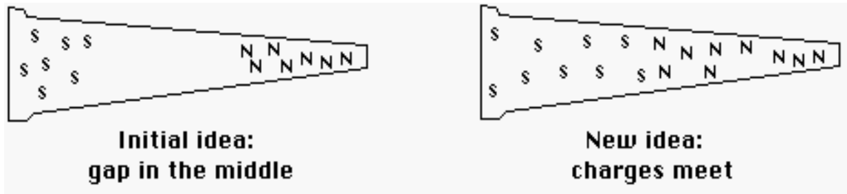
Figure 3: Two models of what might be inside a magnetized nail. The group's original model is represented on the left, with N and S charges separated. Donna's alternate conception is represented on the right.
