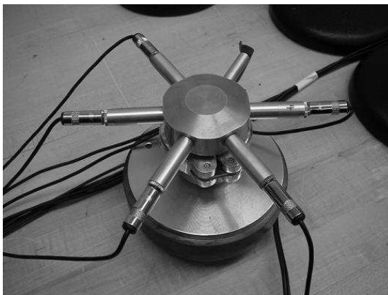
Figure 3.7: The calibration cell holds all six microphones equidistant from the driver. The driver runs through user-defined frequencies at a constant amplitude while the PreSonus collects phasors. These data allow MATLAB to correct for differences in microphone sensitivity.
