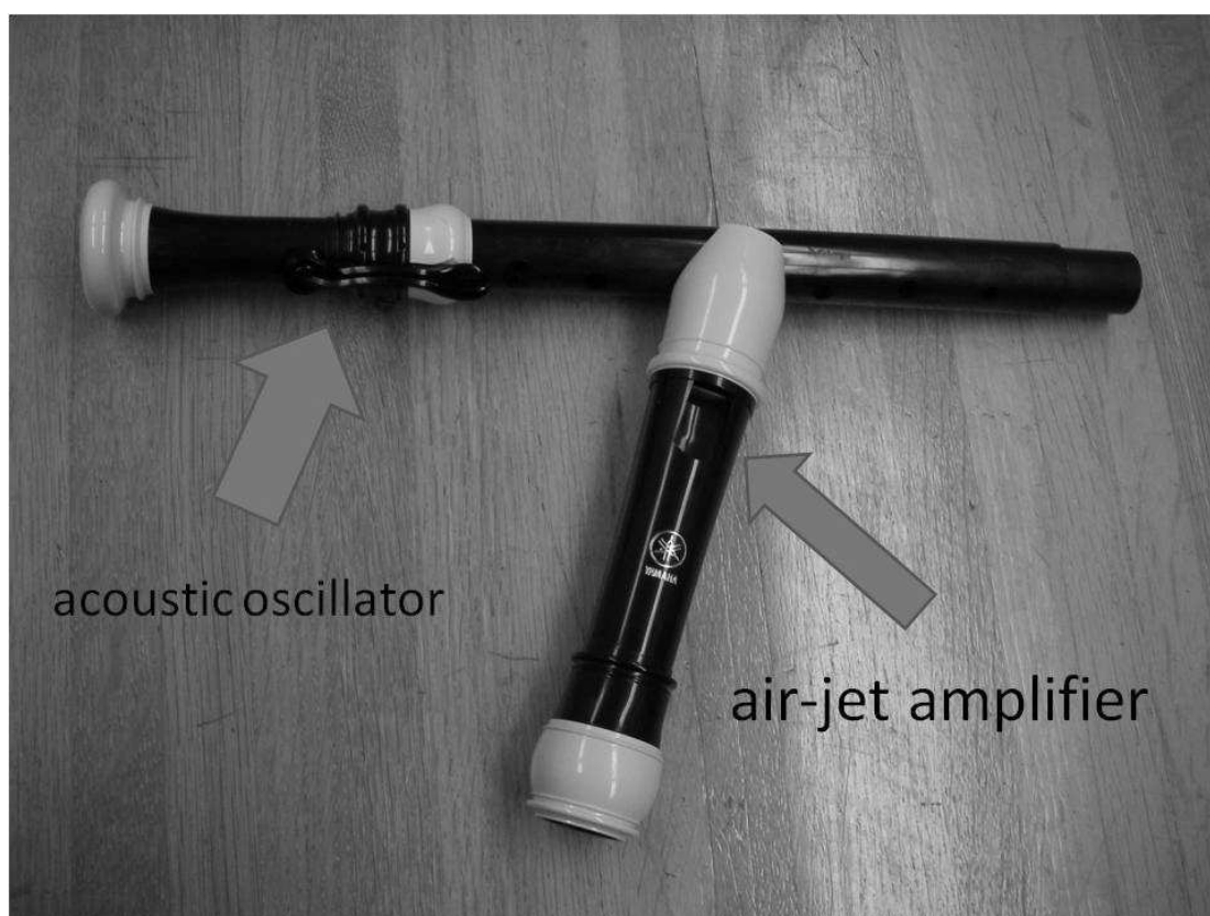
Figure 4.4: This project assumes two simplified elements: an air-jet amplifier and an acoustic resonator.
